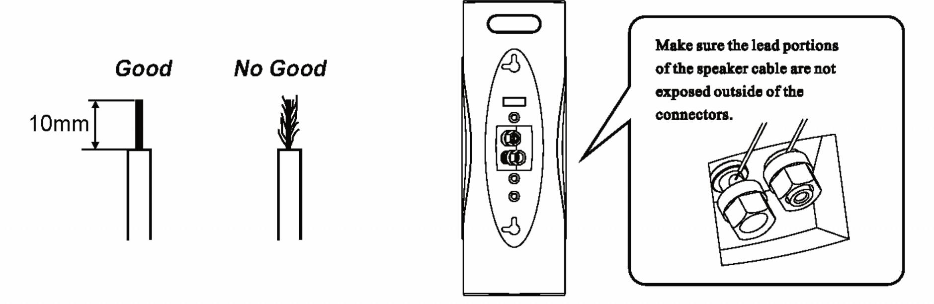
3 Tighten the knob and secure the cord.
